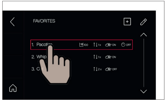
Saved favorites are displayed under Settings > Favorites. The respective parameters can be edited by selecting the recipe.
