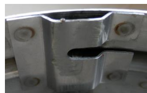
1. The three bayonet slots, identified, locate with the three pins on the black ring shown.
