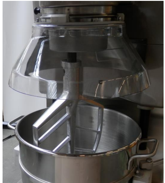
2. Remove the ingredient chute and lower the bowl.
