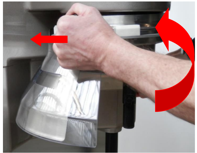
7. Hold the plunger and rotate the guard anti-clockwise to disengage.
