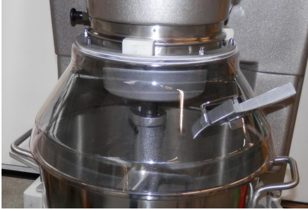
1. Solid dust guard closed with ingredient chute fitted.
