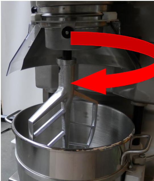
3. Open the guard rotating clockwise/to the left.
