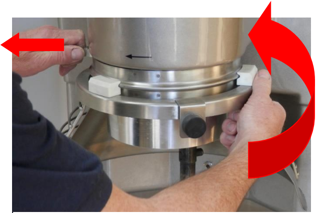
7. Hold the plunger and rotate the guard anti-clockwise to disengage.
