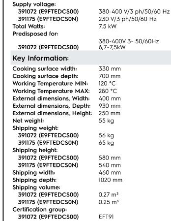
391175 (E9FTEDCS0N) If appliance is set up or next to or against temperature sensitive furniture or similar, a safety gap of approximately 150 mm should be maintained or some form of heat insulation fitted.
