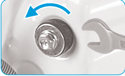
Loosen the 4 transport bolts with a spanner.
