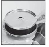
Next, fit the corresponding slicing disc (straightedged blade) and rotate in a clockwise direction to ensure that it is correctly positioned.
