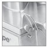
4) Position the head of the vegetable preparation machine on the motor shaft. The fastening hook should now be facing you, on your right.
