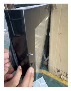
Carefully, put the screw through the hole from inner side. 3.
