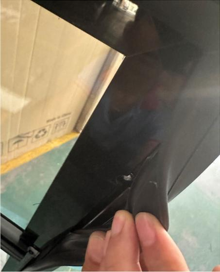
Remove the door seal by hand to reveal the position of the hole.
