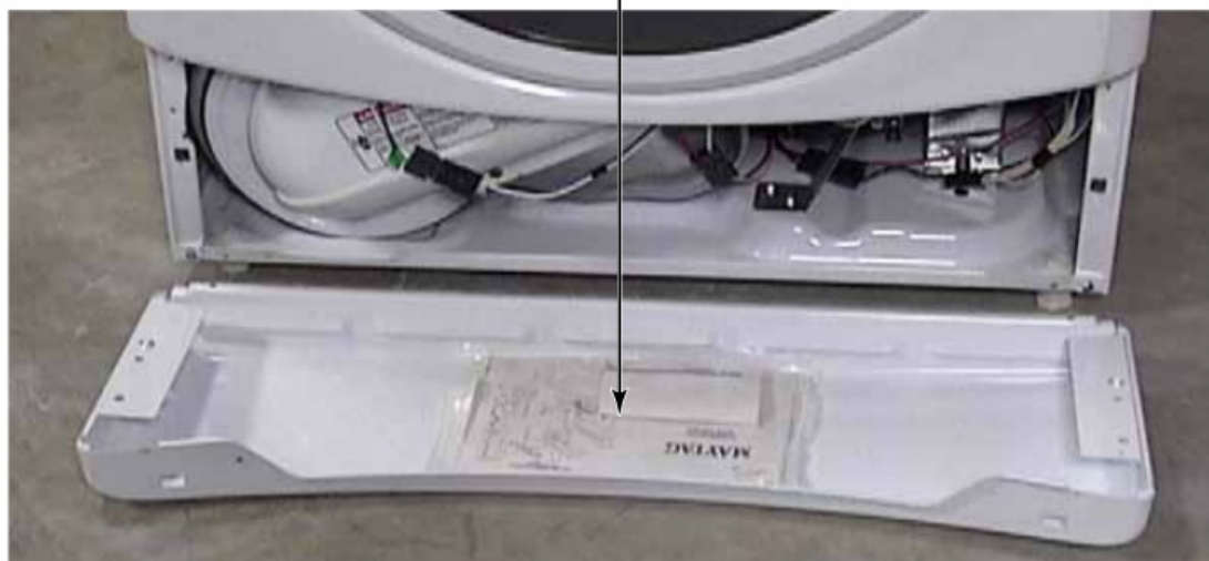
Location of Tech Sheet, Parts List & Wiring Diagram Inside The Service Panel
