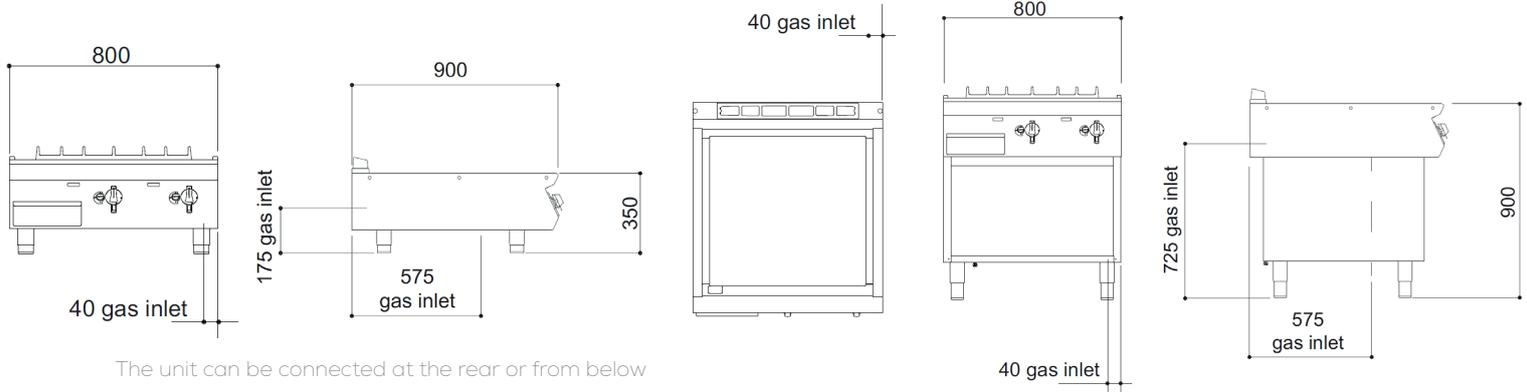
The unit can be connected at the rear or from below
